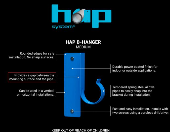
Common Applications HAP System pipe brackets are designed to hold & protect pipes securely and provide protection from nails or screws penetration.
