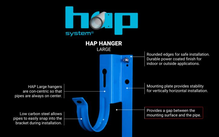
Fast and easy installation. Installs with two screws using a cordless drill/driver.
